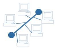
The bus carries packets along the cable. As the packets arrive at each computer system, it checks the destination address contained in the packet to see if it matches its own. If the address does not match, the computer system ignores the packet. If the address of the computer system matches that contained in the packet, it processes the data.
