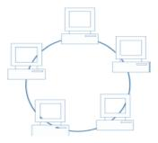
In a ring network, computer systems are connected in a ring or a loop. Packets are sent around the ring, being passed from one computer system to the next until they arrive at their destination.
